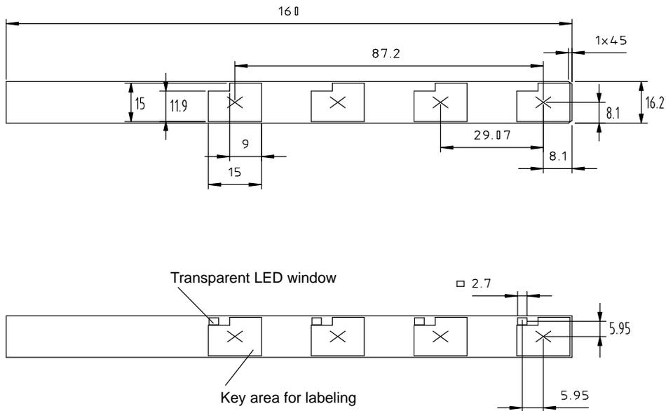
Figure 16-5 Dimensions of Labeling Strips for the OP7
