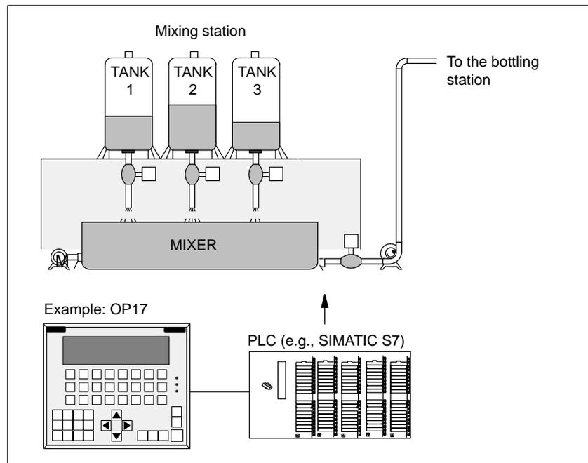
Figure 8-1 Example of a fruit juice plant
