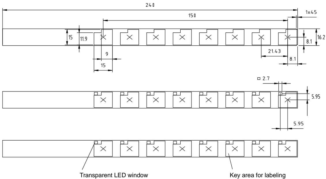
Figure 16-4 Dimensions of Labeling Strips for the OP17
