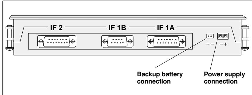
Figure 16-2 Locations of the Connection Elements on the Underside of the OP17
