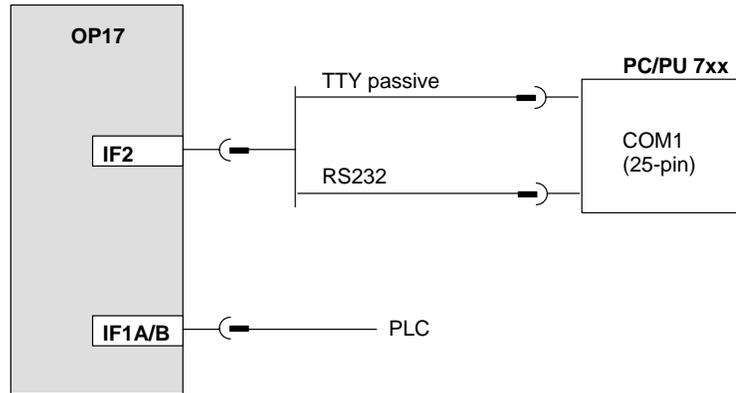
Figure 14-4 Connection Configuration Scheme for AS511 Loop-Through Mode
