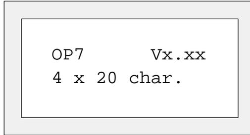
Figure 7-1 Example of Standard Standby Message on OP7
