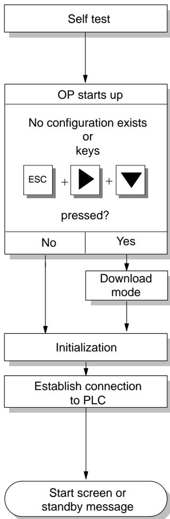
After the power supply has been turned on, the OP performs a self test. In the test, it checks the operability of the most important device components and displays the test results.
