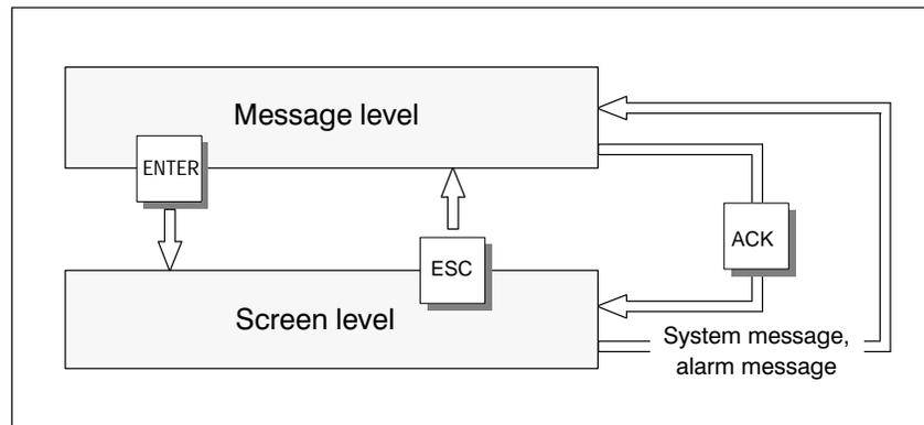
Figure 4-1 Changing between Message Level and Screen Level
