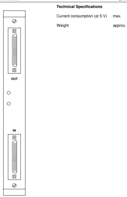
The AS 301 interface module is used in combination with the AS 310 interface module for distributed connection (up to 200 m, or 656 ft.) of expansion units (EUs) to a central controller (CC) (see also Chapter 3).
