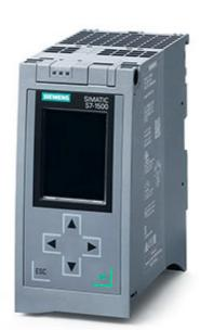
SIMATIC S7-1500F, CPU 1515F-2 PN, Central processing unit with work memory 750 KB for Program and 3 MB for data, 1st interface: PROFINET IRT with 2-port switch, 2nd interface: PROFINET RT, 30 ns bit performance, SIMATIC Memory Card required
