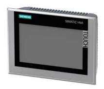
SIMATIC HMI TP700 Comfort INOX, Stainless steel front, Continuous decorative film, Degree of protection front IP66K, 7" widescreen TFT display, PROFINET interface, MPI/PROFIBUS DP interface, 12 MB configuration memory, Windows CE 6.0, (Microsoft Support included Security updates discontinued) configurable from WinCC Comfort V11
