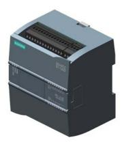
SIMATIC S7-1200, CPU 1212C, compact CPU, DC/DC/DC, onboard I/O: 8 DI 24 V DC; 6 DO 24 V DC; 2 AI 0-10 V DC, Power supply: DC 20.4-28.8V DC, Program/data memory 75 KB
