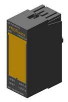
SIPLUS ET 200S EM F-DI 24V PROFIsafe based on 6ES7138-4FA05-0AB0 with conformal coating, -25...+60 °C, electronic module for ET 200S, 4/8 F-DI PROFIsafe, 24 V DC, 30 mm overall width, up to category 4 (EN 954-1)/ SIL3 (IEC 61508)/PLE (ISO 13849), can also be used in PROFINET configuration with IM 151-3 HF
