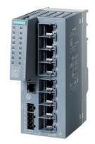
SCALANCE XC208G manageable Layer 2 IE switch; IEC 62443-4-2 certified; 8x 10/100/1000 Mbit/s; RJ45 ports; 1x console port; diagnostics LED; redundant power supply; temperature range -40 °C to +70 °C; assembly: DIN rail/S7 mounting rail/wall redundancy functions; office features (RSTP, VLAN,...); PROFINET IO device; Ethernet/IP-compliant; C-PLUG slot;
