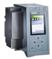
\*\*\*spare part\*\*\* SIPLUS S7-1500 CPU 1516-3 PN/DP based on 6ES7516-3AN01-0AB0 with conformal coating, -40...+70 °C, start up -20 °C, heat sink, no PS usable, central processing unit with work memory 1 MB for program and 5 MB for data, 1st interface: PROFINET IRT with 2-port switch, 2nd interface: PROFINET RT, 3rd interface: PROFIBUS, 10 ns bit performance, SIMATIC Memory Card required
